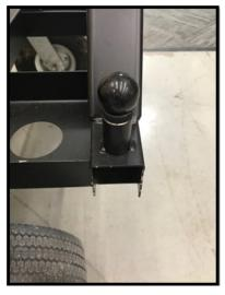
Spring pin and receiver for outriggers
